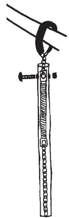
**Figure 7. Small-diameter PVC encases a garage door spring to prevent a tiger’s claws, lips, etc. from becoming trapped in the spring. The PVC is twice the length of the spring so that even if fully extended, the spring is entirely inside the PVC (Hare and Jarand, 1998).**
